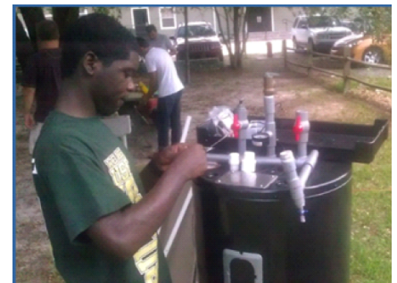
Herby Jean checking fittings for an anaerobic biodigester
